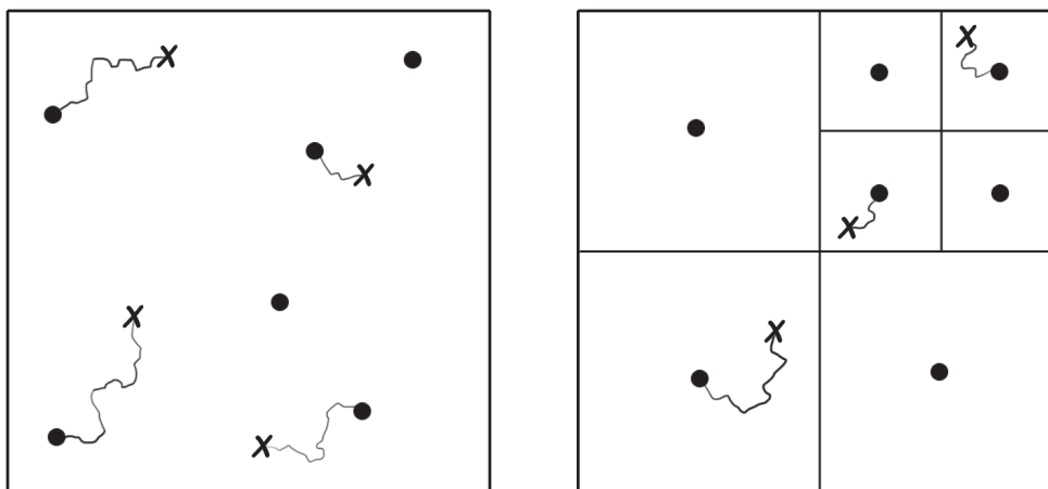
Figure 38.14: Different ways of allocating local searchers: by Memetic Algorithms (left) and by a political analogy (right). Crosses represent starting points, circles local optima reached after running local search. In the second case each individual is responsible for an area of configuration space. The political analogy is with territorial subdivisions given by electoral districts, or areas assigned to different marketing managers in a business example. Some local search streams are shown.
